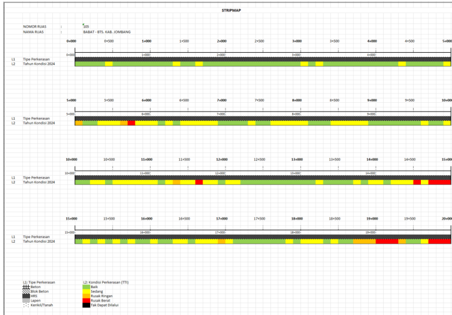
Figure 1. Example of Strip Map Results for the Babat - Bts Road Section. Jombang Regency
