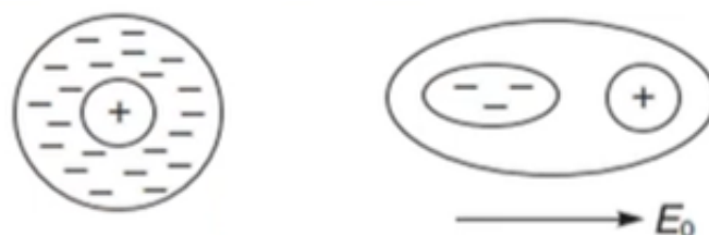
Figure.2. Electrical polarisation phenomenon in dielectric materials
