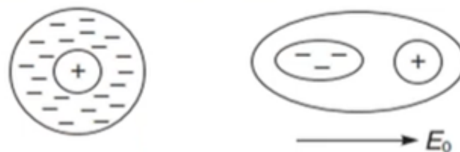
Figure.2. Electrical polarisation phenomenon in dielectric materials
