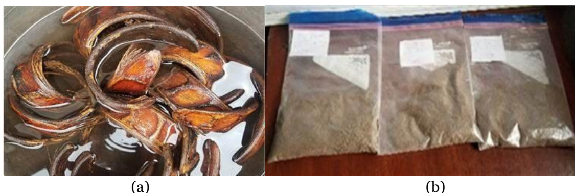
Figure 1. (a) Washing of empty fruit husk (b) Milled and dried fruit husk fibres
