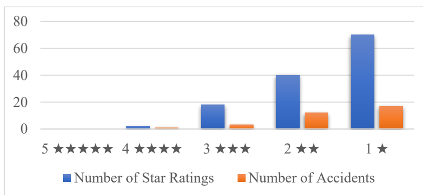
Figure 6. Relationship Between iRAP Star Rating and Accident Frequency
