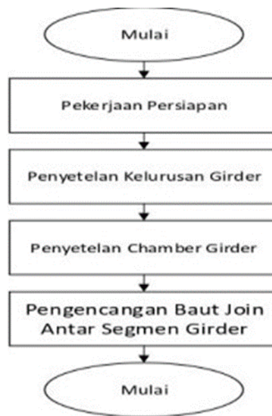
Figure 3. Flowchart of steel box girder ground assembly Source: Wika-Nindya KSO Implementation RKK Document
