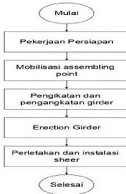
Figure 1. Flowchart of steel box girder erection implementation
